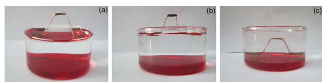
Figure 4. Optical images for the artificial strider (a and b) floating on the water surface and (c) at the water/ \text{CHCl}_3 interface. The \text{CHCl}_3 layer was dyed red by Rhodamine B for clear observation.
